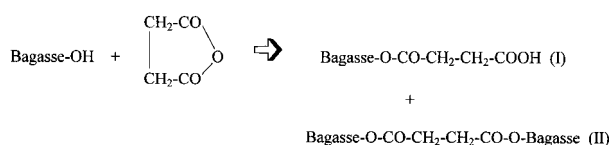
Figure 4 Reaction scheme between with bagasse fiber constituents and succinic anhydride.
